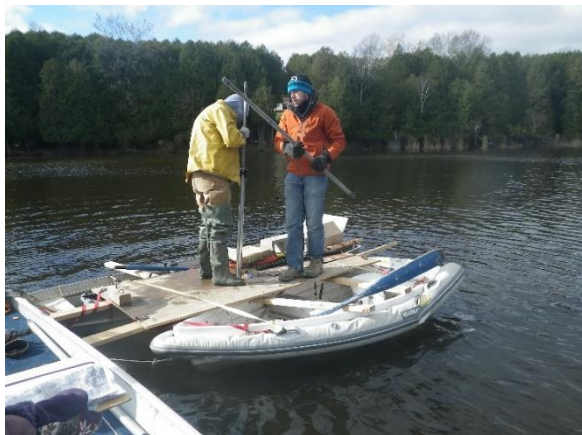
Figure 6-2. Sediment Core Collection
